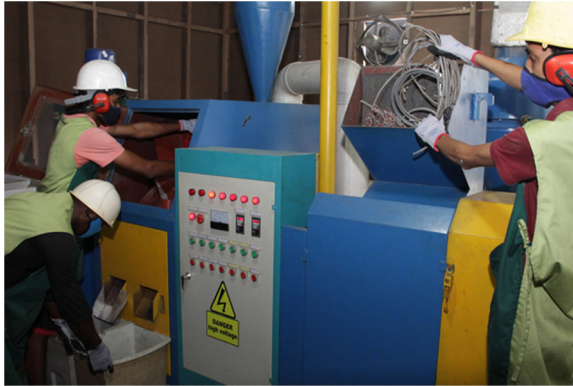
Figure 13.5 Splitting cables in a formal sector dismantling facility.
