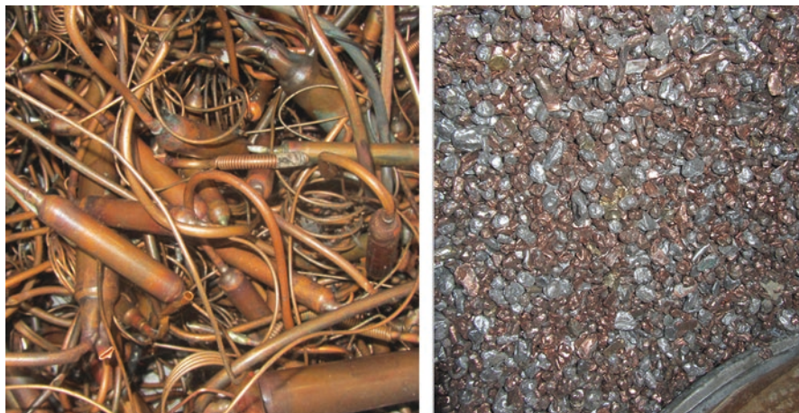
Fig. 2.3 Copper components from manual disassembly (left) and copper fraction from the processing line. This material comes from refrigerators and cooling appliances
